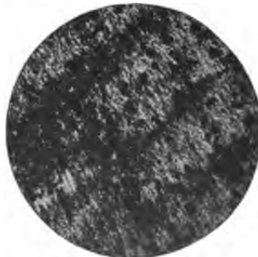
Fig. 26. Temper drawn at 550 Degrees C.; Sorbite Structure
